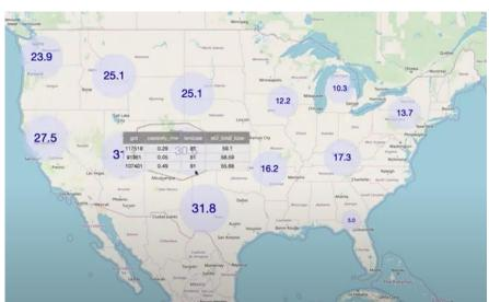
In the image above, the blue dots represent total capacity within that wide area; users can drill down into each area to reveal additional detail down to a single turbine in its specific geolocation.
